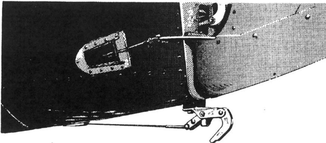
**FIGURE 8-5. CONVENTIONAL GEAR AIRCRAFT-LEAF SPRING TYPE TAILWHEEL**
