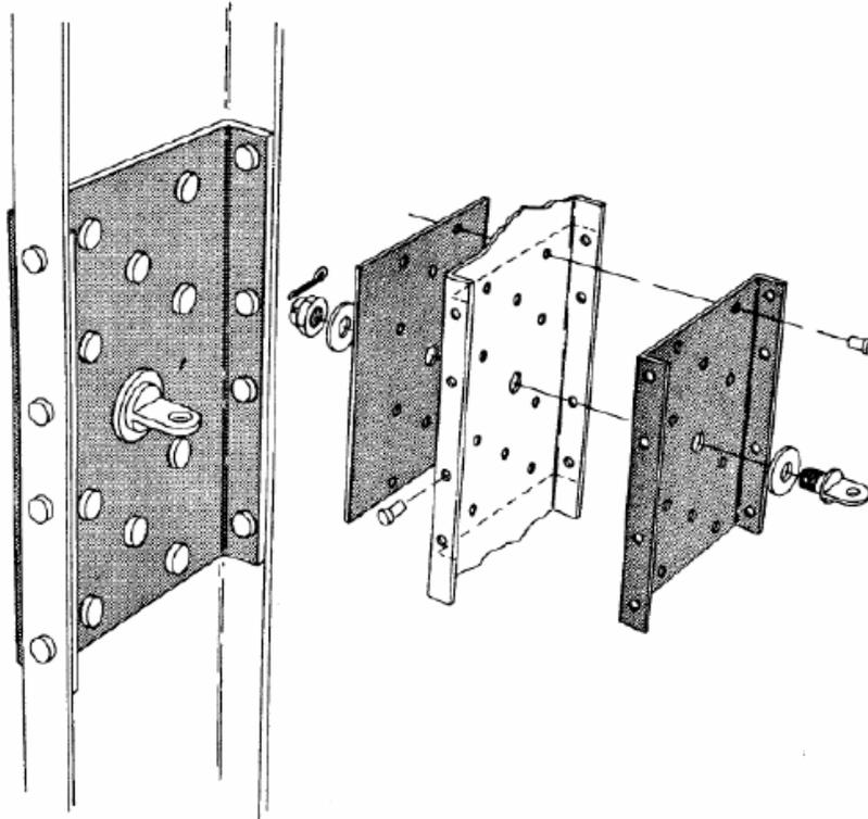
**FIGURE 9-17. TYPICAL STRINGER SECTION REINFORCEMENT INSTALLATION**
