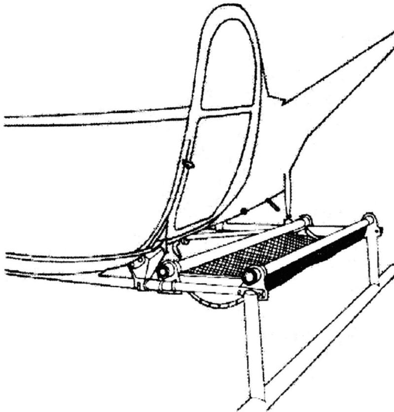
**709. STATIC TEST.** The cargo rack installation must be able to withstand the static test load required by § 133.43(a). Conduct the test as outlined in chapter 1.
