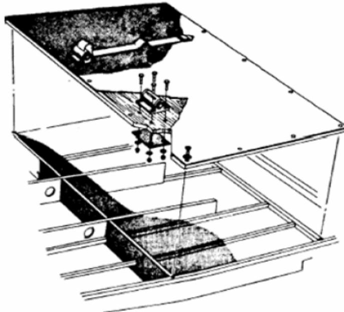
**FIGURE 9-13. TYPICAL SEAT MOUNTED INERTIA REEL INSTALLATION**
