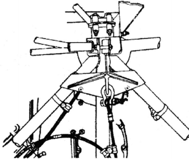
**FIGURE 7-5. TYPICAL CARGO SLING INSTALLATION NO. 1
