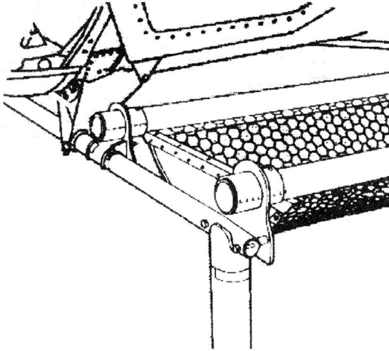
**FIGURE 7-12. TYPICAL CARGO RACK INSTALLATION NO. 2**
