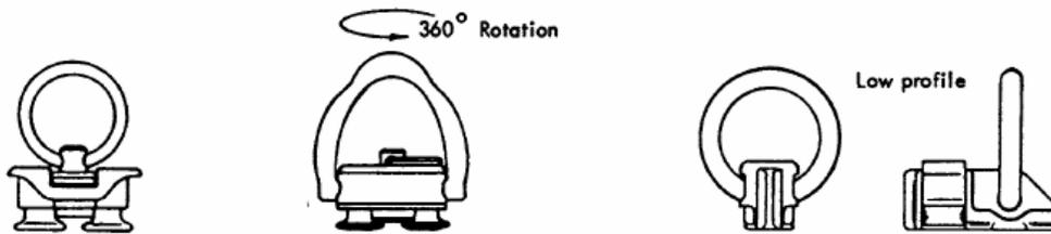
These types of cargo tie down fittings are of greater capacity than the single pin types and are suitable for use with the extruded track style shown above.
