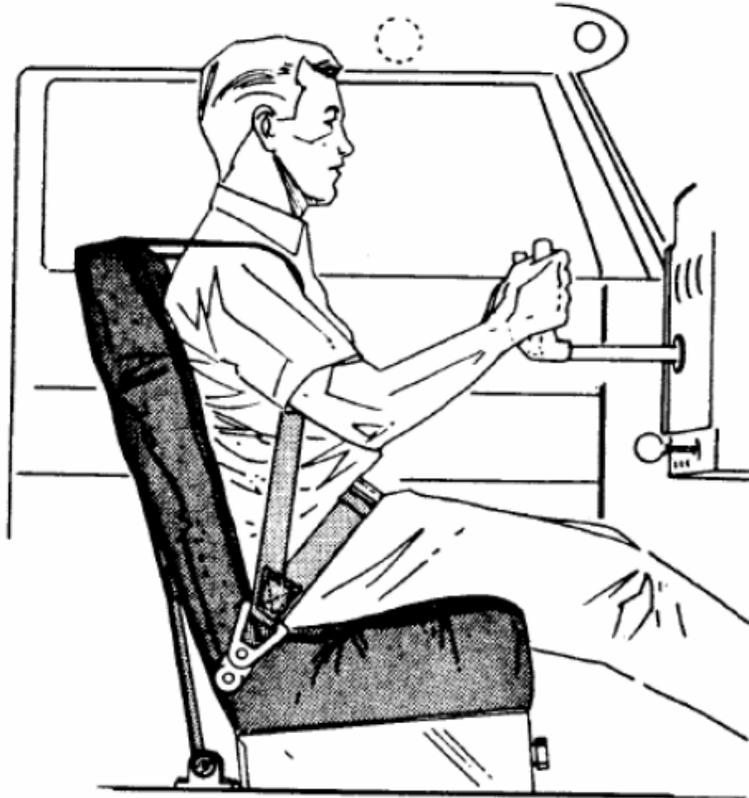
**FIGURE 9-12. TYPICAL FLOOR MOUNTED INERTIA REEL INSTALLATION**
