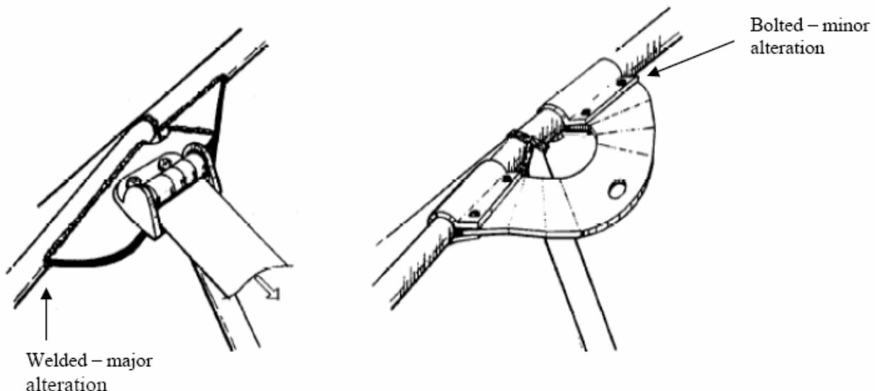
**904. RESTRAINT SYSTEM CONFIGURATIONS.** Restraint systems incorporating a shoulder harness are available in three configurations:
