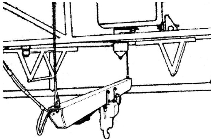
**FIGURE 7-6. TYPICAL CARGO SLING INSTALLATION NO. 2 (CARGO HOOK ATTACHED DIRECTLY TO UNDERSIDE OF FUSELAGE)**
