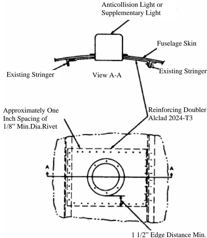
**b.** When a formed angle stringer is cut and partially removed, position the reinforcement doubler between the skin and the frame. The doubler is to be equivalent to the stringer in thickness and extend lengthwise beyond the adjacent fuselage frames. The distance between the light and the edge of the doubler is to be twice the height of the doubler flange. (See Figure 4-2 for typical installation.)
