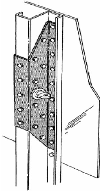
**FIGURE 9-19. TYPICAL ATTACHMENTS TO TUBULAR MEMBERS**
