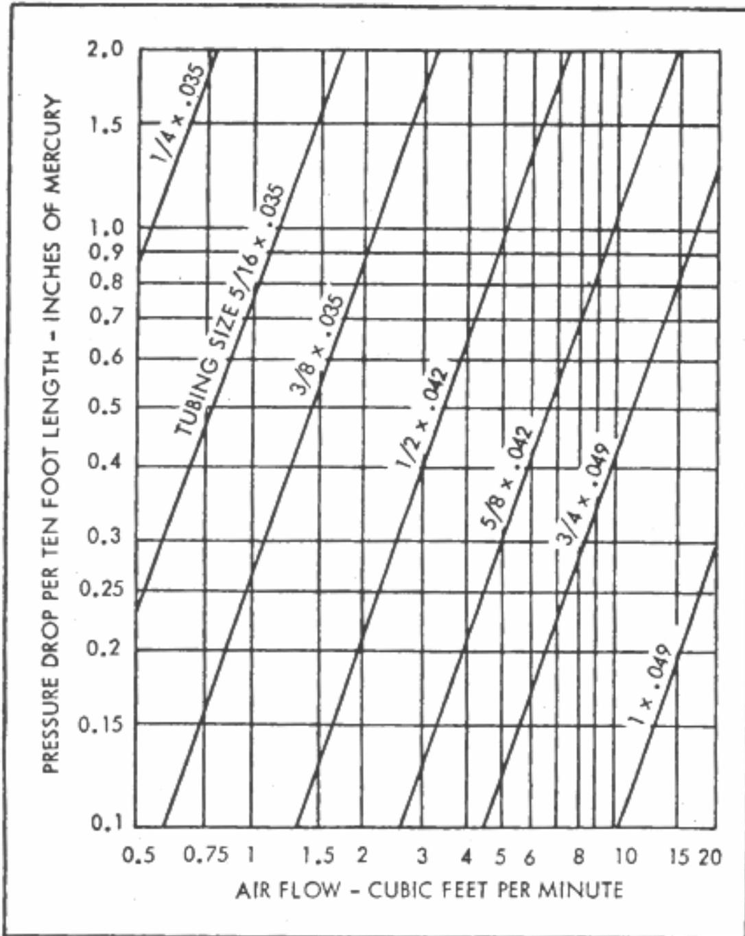
1. The pressure drop for each 10-foot length of that tube is 0.68" Hg.
