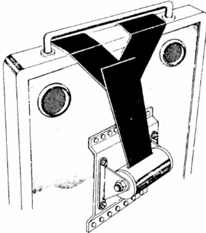
**b. Airframe Attachments.** The method used for the attachment of shoulder harness anchorages is dependent upon the construction features of the aircraft involved. When selecting a point of attachment, careful consideration should be given to the static strength and testing requirements found in section 3.
