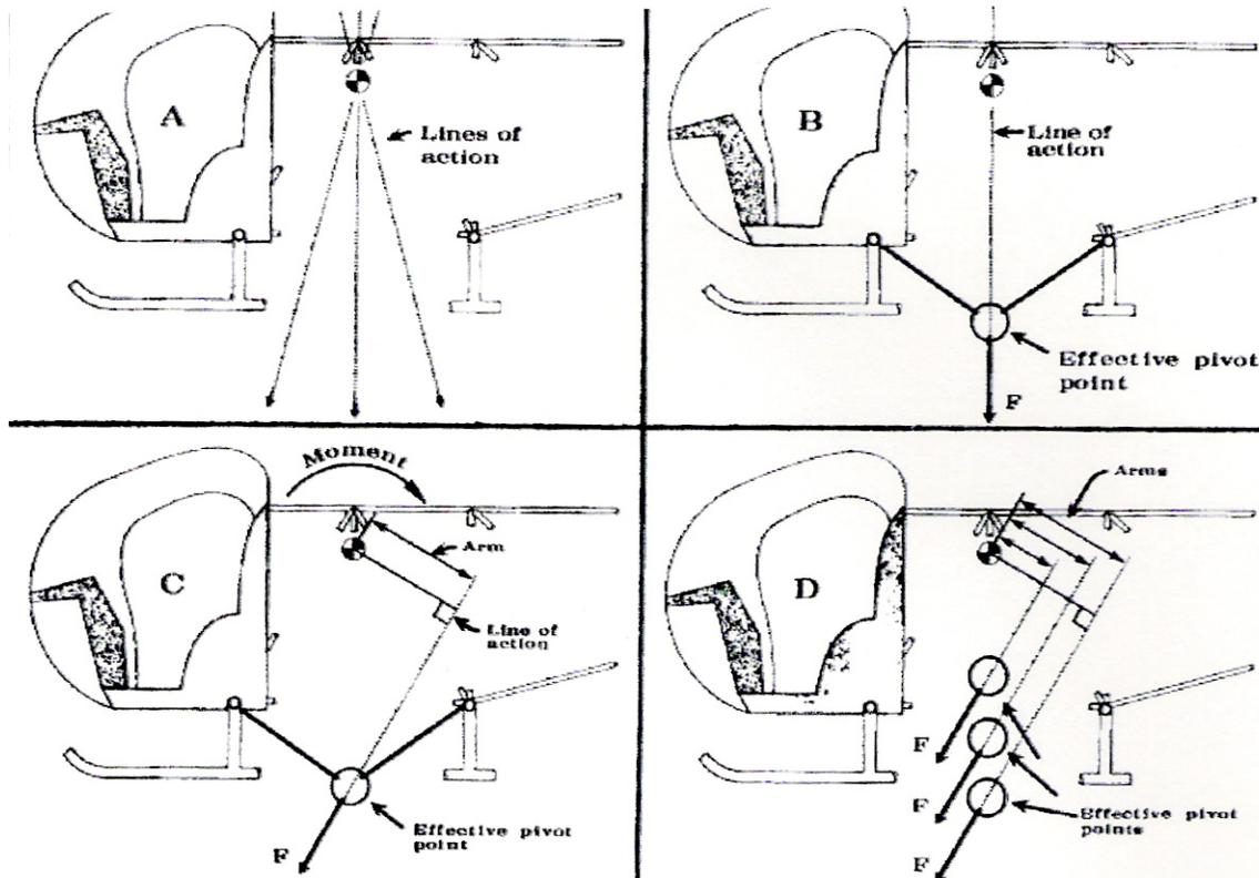
(2) Thus, any attachment method or location which will decrease the length of the arm will reduce the distance that the combined CG will shift for a given load ( $F$ ) and line of action angle. (See Figure 7-1, Illustration D.)
