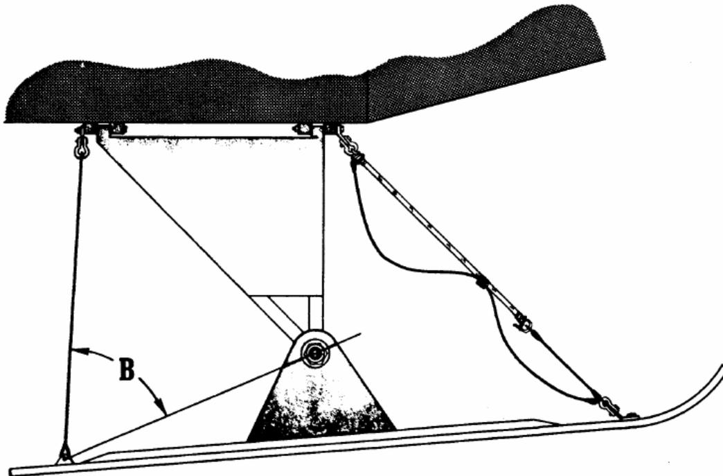
**a. Location of Attach Fittings on Fuselage or Landing Gear.** Locate fittings so the shock cord and cable angles are not less than 20 degrees when measured in the vertical plane with the shock absorber in the fully extended position (see Angle B, Figures 5-4 and 5-5).
