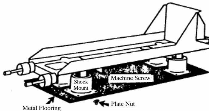
**b. Rigid-Mounted Unit Base.** Secure radio mounting base plate(s) to the floor (wood, composite, or metal) using machine screws as shown in Figure 2-6. Use a reinforcing plate or large
