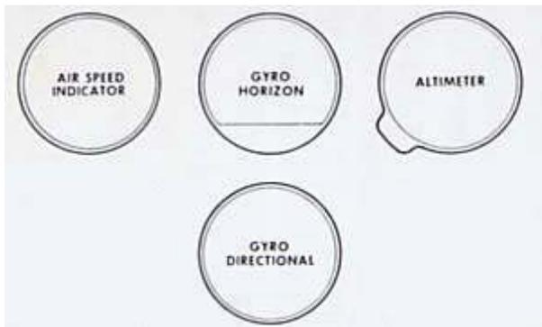
(1) The aircraft attitude indicator is located at the top center of the installation.
