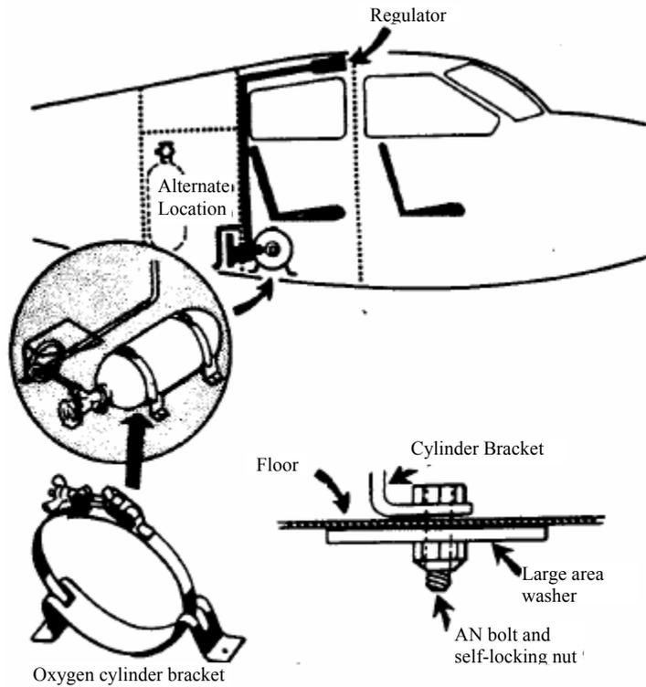
Reinforce floor, if necessary, to withstand the added load.
