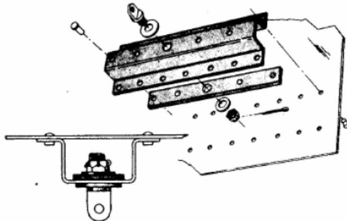
**FIGURE 9-16. TYPICAL BULKHEAD REINFORCEMENT INSTALLATION**
