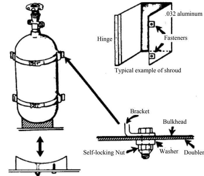
Cylinder support block – Cut to fit contour of cylinder base.
