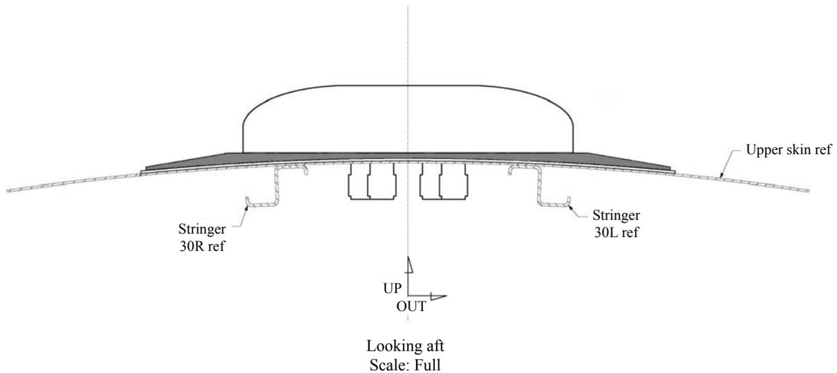
**d.** Mounting screws must never be over torqued in an attempt to distort aircraft structure to reduce gaps between the antenna base plate and aircraft-mounting surface.
