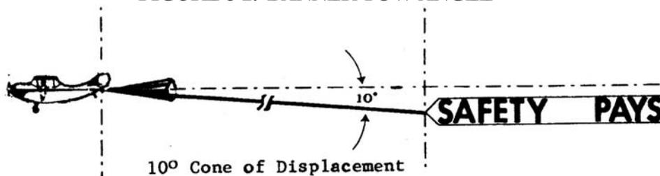
(2) Another approach can be applied if the limit load carrying capabilities of a tow hook and fuselage are known. In this case, the known load value can be divided by 1.5 to arrive at the design load limits. For example, if the tow hook and fuselage limit loads are known to be 1,800 pounds,
