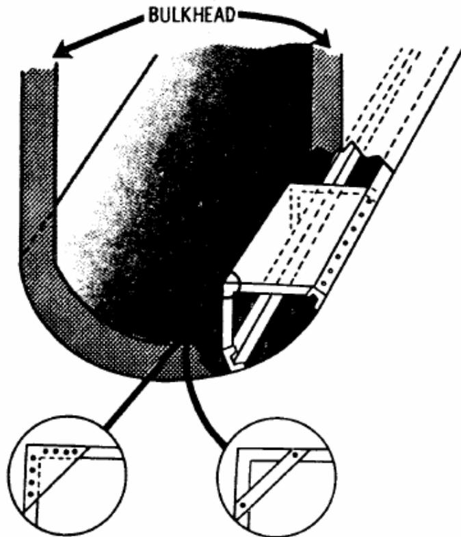
**NOTE:** Use standard aircraft practices and procedures for fabrication and attachment of the shelf. Reinforce fore and aft corners with gussets or bulb angle.
