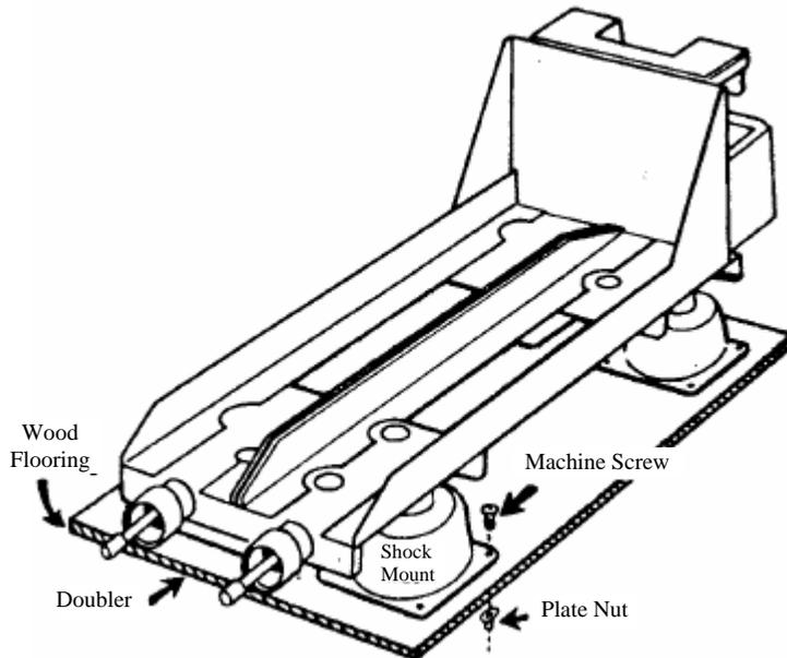
(2) **Metal Flooring.** Secure the shock-mounted base assembly directly to the floor using machine screws, washers, and self-locking nuts. Floor area under and around the radio mounting bases may require installation of doublers or other
