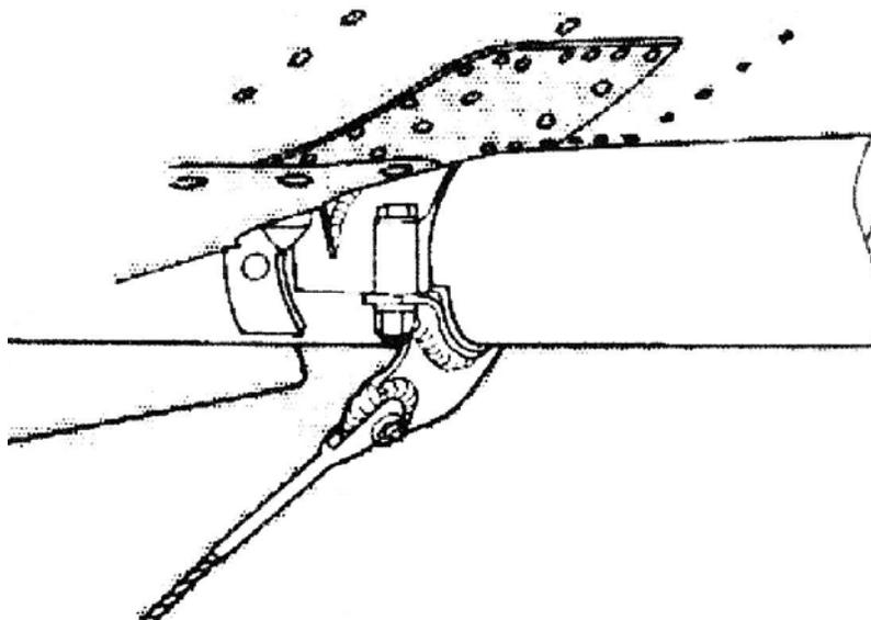
**FIGURE 7-9. TYPICAL CARGO SLING INSTALLATION NO. 3 (SHOWING CARGO SLING IN STOWED POSITION)**
