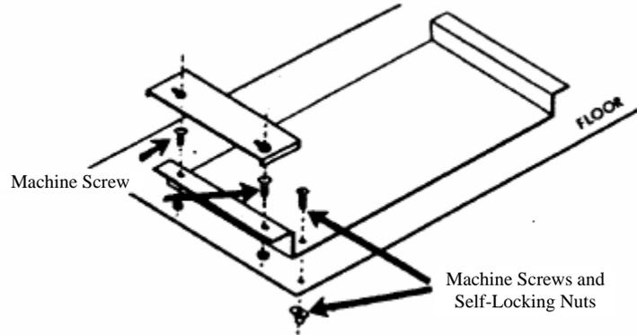
**205. FABRICATION OF SUPPORTING BRACKETS FOR ATTACHMENT TO STRUCTURE OTHER THAN FLOORING.**
