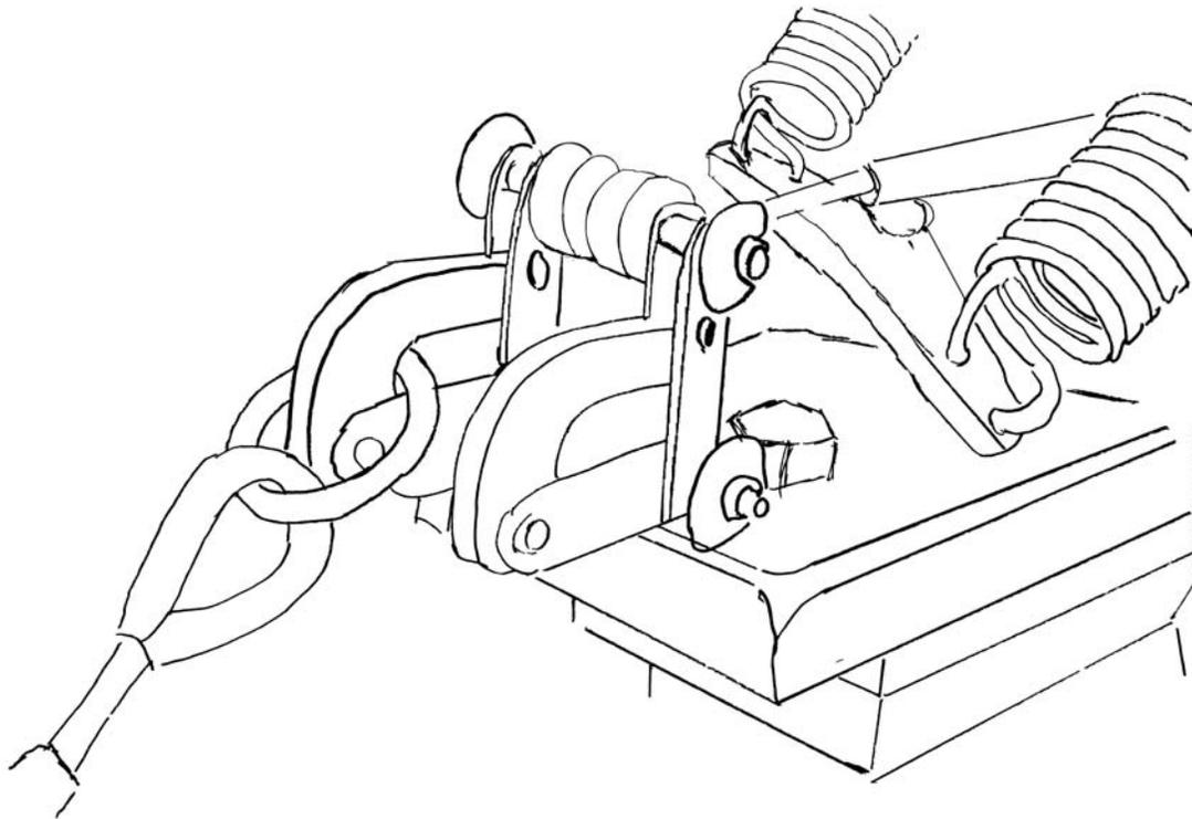
**FIGURE 8-12. TYPICAL TOST MOUNT FOR TRICYCLE GEAR AIRCRAFT**
