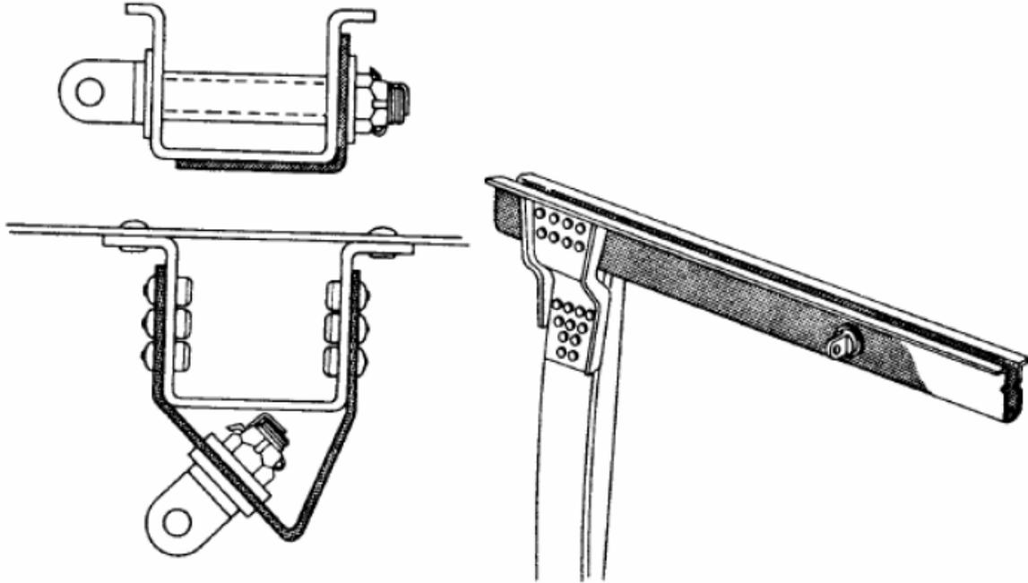
**FIGURE 9-15. TYPICAL HAT SECTION REINFORCEMENT INSTALLATION**
