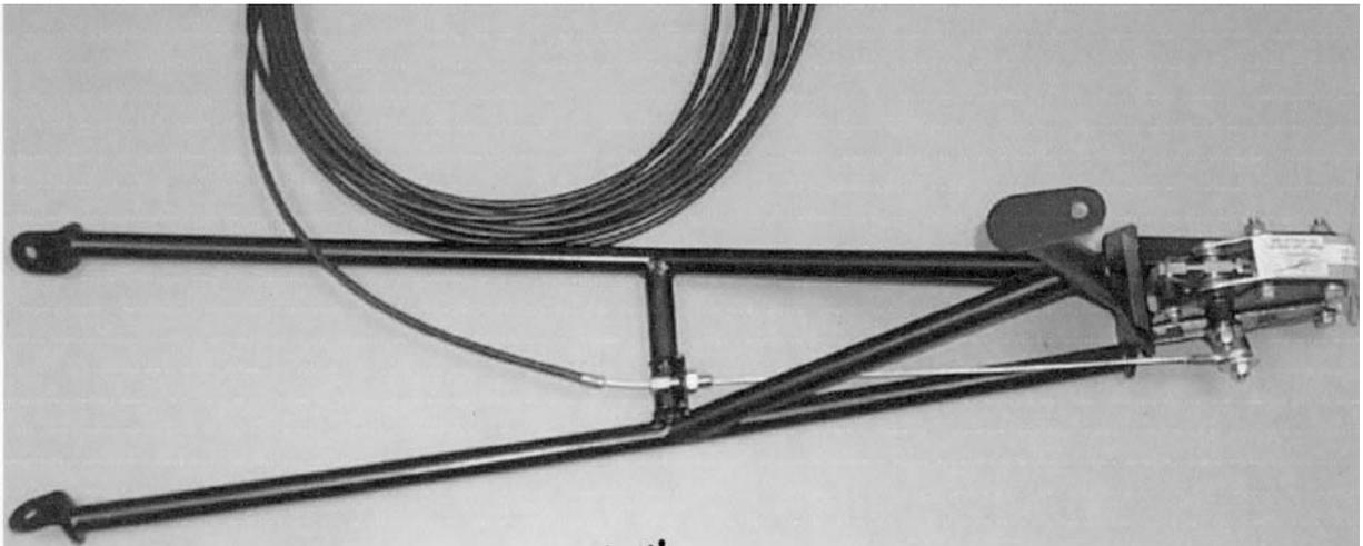
**FIGURE 8-13. TYPICAL TOST CONVENTIONAL LEAF SPRING MOUNT**
