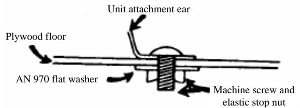
**NOTE: To increase the strength of floor attachment points, metal reinforcement may be installed as needed.**
