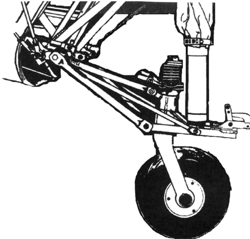
**FIGURE 8-7. CONVENTIONAL GEAR AIRCRAFT – TUBULAR SPRING TYPE TAILWHEEL**
