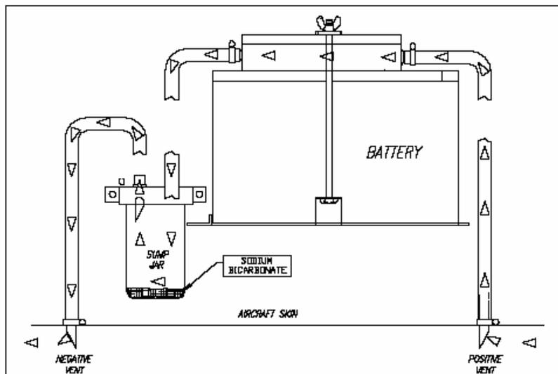
**b. Free Airflow Type.** Battery cases or boxes that contain louvers may be installed without an individual vent system, provided that:
