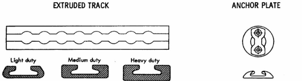
Extruded track and anchor plates are available in several different styles and load capacities and will accommodate a wide variety of quick attachment fittings.
