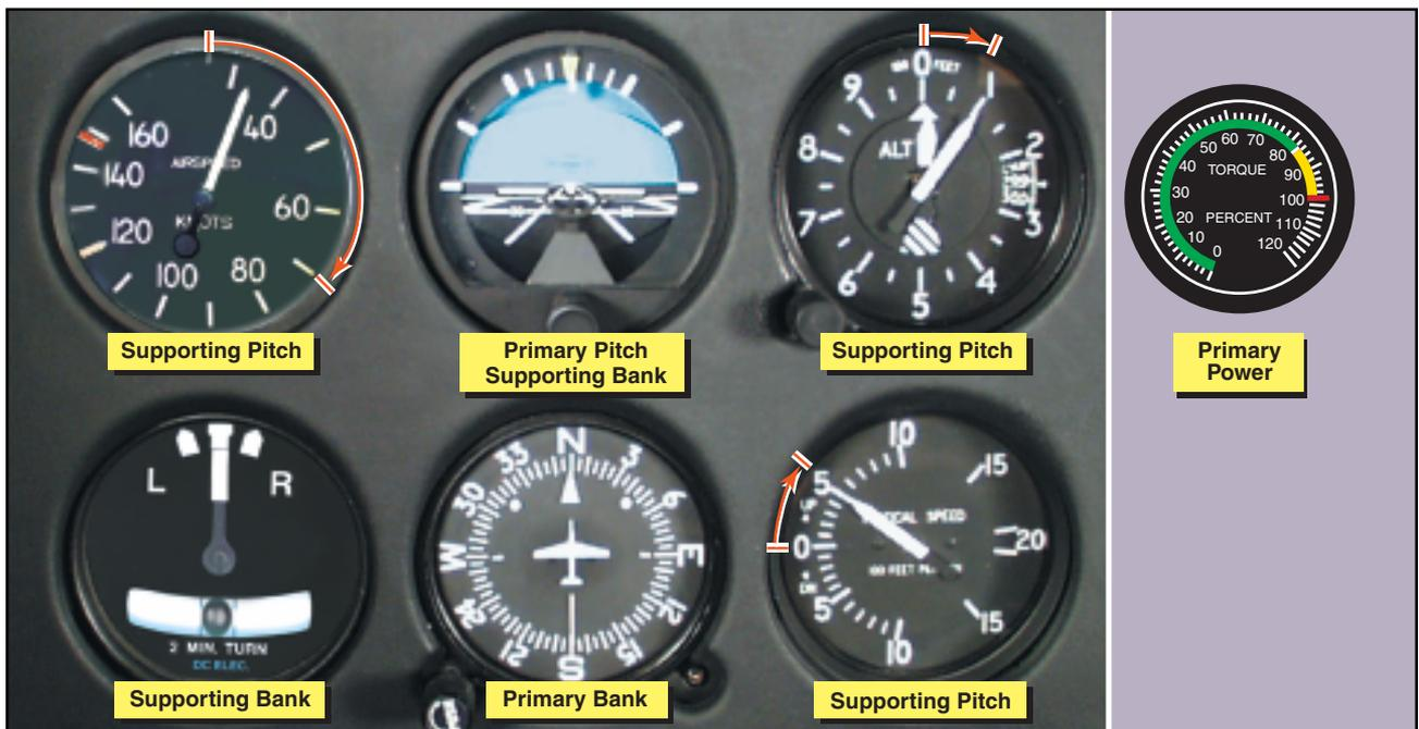
Figure 12-22. Flight instrument indications during an instrument takeoff.
