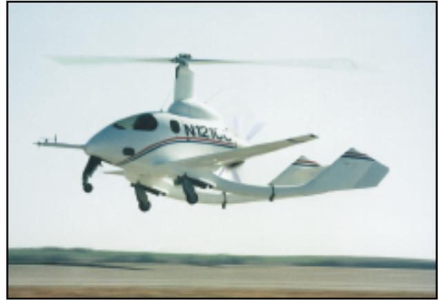
**Figure 15-3. The CarterCopter uses wings to enhance performance.**
